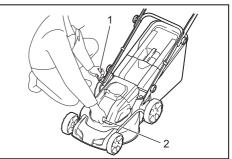
1. Mowing height adjusting lever 2. Front grip
