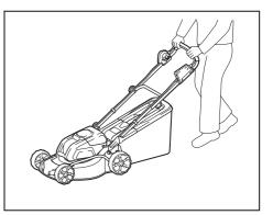
The center lines of the front wheels are guidelines to mowing width. Using the center lines as guidelines, mow in strips. Overlap by one half to one third the previous strip to mow the lawn evenly.
