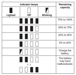
**NOTE:** Depending on the conditions of use and the ambient temperature, the indication may differ slightly from the actual capacity.
