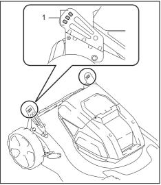
**NOTE:** The handle height can be adjusted in three levels by replacing the bolt in one of the three holes on each side of the mower body. For details, refer to the section for adjusting the handle height.
