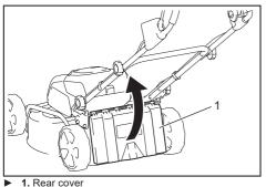
2. Remove the mulching attachment while holding
