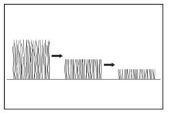
**NOTE:** Mowing long grass to a short length all at once may cause the grass to die. The cut grass may also block up inside of the mower body.
