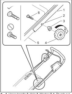
1. Upper handle 2. Hole 3. Washer B 4. Thumb nut
