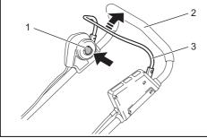
Switch button 2. Upper handle 3. Switch lever
