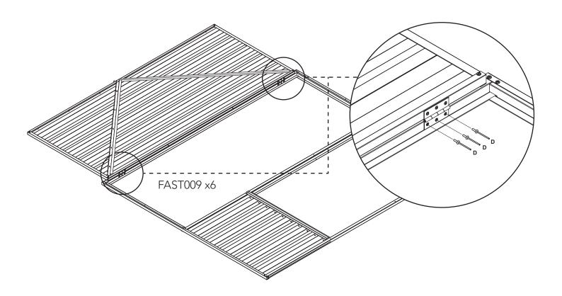
Lay the LEFT SIDE PANEL face up and lay the DOOR PANEL down in the open position on top as shown.
