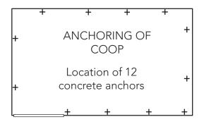
Each anchor consists of one nut, bolt, M10 dynabolt and steel angle.
