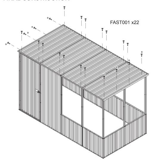
Position the roof so that the back wall has the lip trim against it with the roof overhang to the front.
