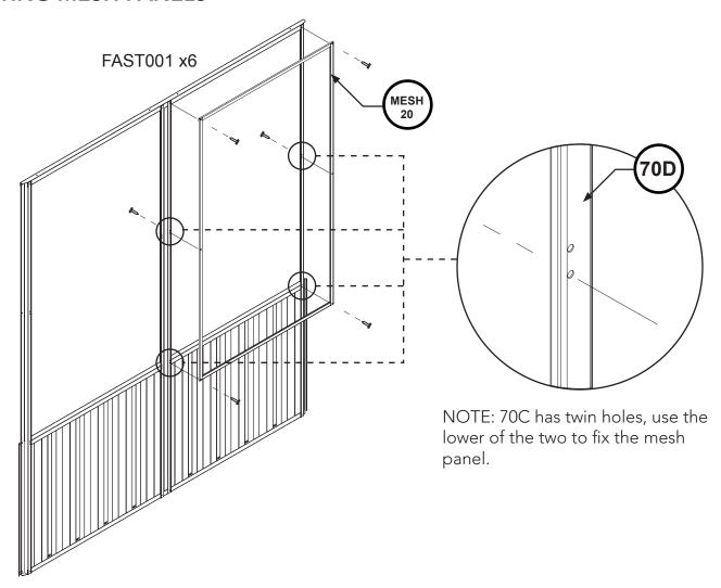
The mesh panels are fixed to the interior of the wall panels.
