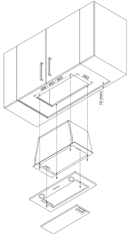
Install Range Hoods in accordance with the manufacturer's instructions. Technika recommends that all Range Hood clearances be a minimum of 650mm to a maximum of 750mm (between the top of the cooking surface and to the underside of the rangehood).
