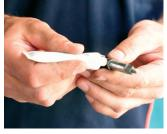
Replace the body washer, the o-ring and the jumper valve with new parts. Apply a tap lubricant to the spindle and valve for better sealing and smoother tap operation.
