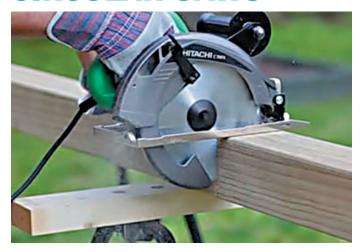
Probably the most common saw found in Australian homes, the circular saw is enduringly popular for its ability to cut pieces of wood to size. Use it to slice neatly through MDF, plywood, kitchen benchtops and decking — and slash the time spent preparing for your next timber construction, whatever it may be.
