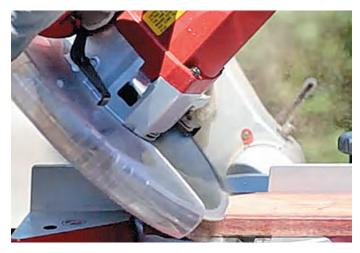
In the same family as the circular saw, the mitre saw offers a few more features and generally offers more precision. It can make cross, mitre and bevel cuts in hardwoods and softwoods, plastic and metals. With this in mind, a mitre saw is great for making picture frames or cutting mouldings or window frames around the home.
