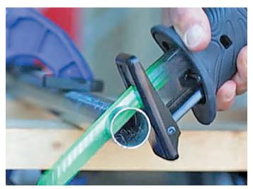
Meet the workhorse of power saws. The reciprocating saw is very popular with more serious DIYers that have a demolition job coming up; or with gardeners that need to do some hard-core branch lopping. These saws are great for cutting overhead, vertically or in tight spaces.
