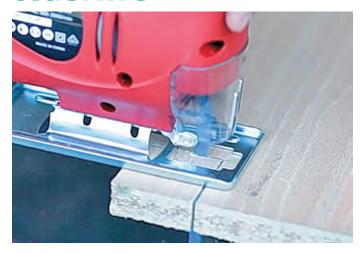
A jigsaw is a great all-rounder when it comes to power saws. It can cut curves, shapes, angles and straight lines in all sorts of materials – like metal, wood, plastic, ceramic, glass, masonry and plaster.
