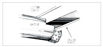
Fit any remaining rafters to the flat sections of the pergola by square cutting at both ends, then notching for the gutter.
