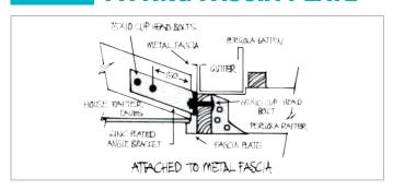
Slide back the tiles and place the bracket against the rafter and inside of the fascia, then mark its position. Drill both holes through the rafter and finally bolt the bracket into place.
