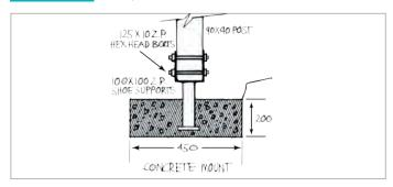
Check to ensure the structure is plumb and level then concrete posts into position and allow to cure before proceeding to the next stage.
