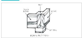
Use the level string line as a reference when calculating post lengths. You should also consider any fall the pergola may need for water run off if you intend to cover it. Measure, mark and cut posts to their appropriate lengths. Our first posts support both fascia beam and beam. Measure down to the height of the fascia beam and draw a line across the post. Then draw a line down the post 30mm in from the side.
