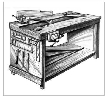
It's easy to go on and customise your new workbench by adding optional end tool boards. Simply cut 2 pieces of pegboard about 810mm wide x 620mm high and screw them to the frames at each end. Now hang your tools on spring clips or pegboard hooks in neat order and mark their outline with a felt pen to make it easy to replace them where they belong. You will also be able to see at a glance what's missing or who hasn't put something back after borrowing it!
