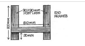
Cut 4 x 800mm lengths from the 90 x 90mm timber. These will be the legs for the bench. Loosely bolt or screw a piece of 90 x 45 x 810mm previously cut timber across the bottom of each pair of legs, at 90mm from the bottom or floor level.
