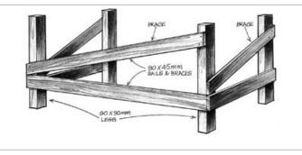
Trim the bracing pieces to length by sawing flush with the outside of the legs once fixed in place.
