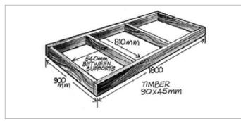
Construct the frame for the bench top first, by cutting  $2 \times 1800$ mm and  $4 \times 810$ mm lengths of the  $90 \times 45$ mm timber. When cutting several pieces of timber to the same length like this, clamp them together all square at one end, then measure and mark the top
